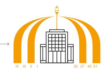
The level of protection is given using NFC 17-102 ed. 2011, or EN 62305-2, or using the FDC 17-108 guide. If the site presents a risk for the environment the protection radius must be reduced of 40%. For a level of protection I++ [cf. 5.2.3.5 NFC 17-102], the radius of protection must be reduced of 40%
